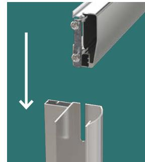
**STEP 1:** Align the horizontal and vertical shower door profiles so they sit straight and upright.
